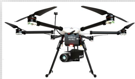
Methane gas leaks detection on the drone platform
