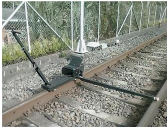
Figure 1-3: Hand pushed tribometer for measuring the coefficient of friction on the rail surface [14]
