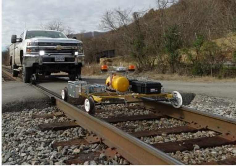
Figure 3-11: Third Generation Rail Lubricity Sensor and Remote Control (RC) Rail Cart in operation during field testing
