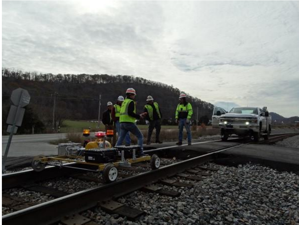
Figure 1-4: Remote Control (RC) Rail Cart and Third Generation Rail Lubricity Sensor setup on track and ready to begin field testing on revenue service track
