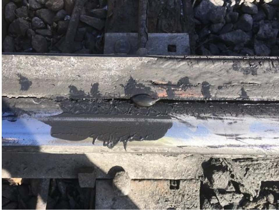
Figure 5-21: TOR wayside applicator functioning correctly in the field with TORFM applied to the rail surface.
