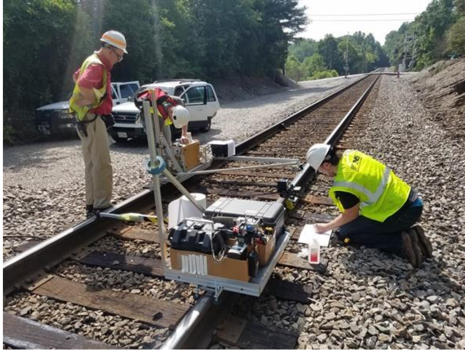
Figure 1-5: Field Testing with Rail Push Cart and Second Generation Rail Lubricity Sensor in the summer of 2018
