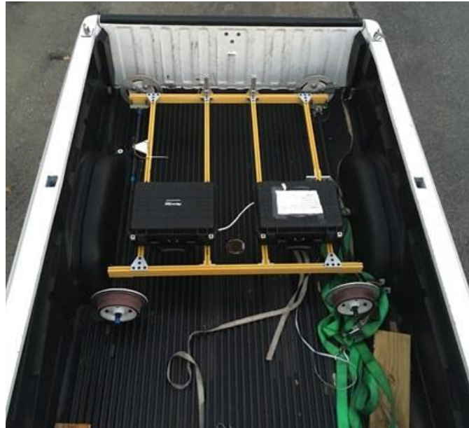
Figure 4-2: Test fit of remote control rail cart in the bed of the lab pickup truck
