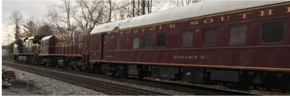
Figure 4-5: An example of a track geometry train operated by Norfolk Southern. Photo taken with permission.
