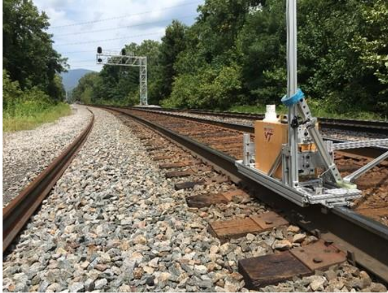
Figure 3-3: Second Generation Lubricity Assessment System in operation during moving field testing [4]
