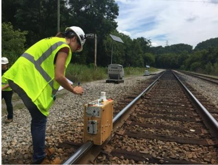
Figure 3-2: Second Generation Rail Lubricity Sensor in operation during field testing [31]
