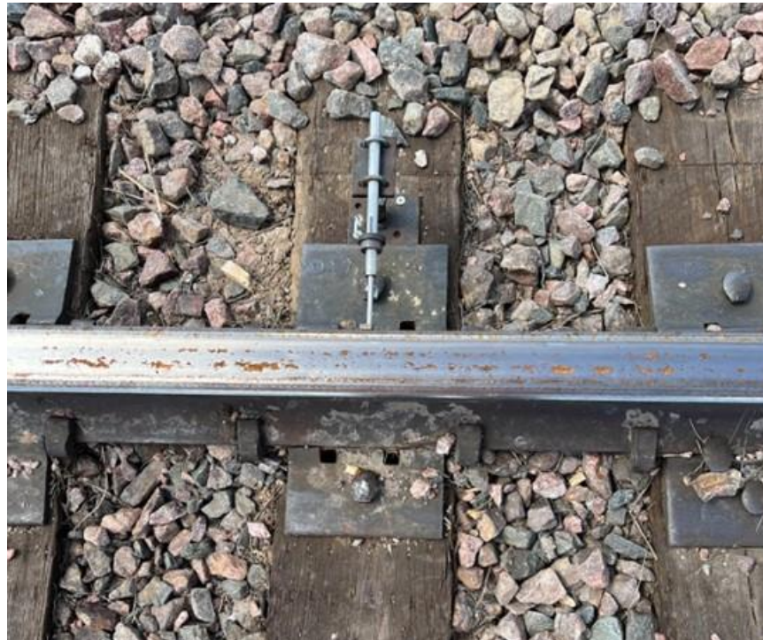
Figure 4-1: Fish scales mounted on the tie to measure the lateral deflection of the rail
