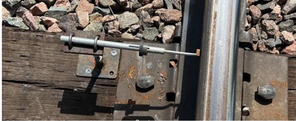
Figure 2-5: A fish scale connected to field side gage face of the rail.
