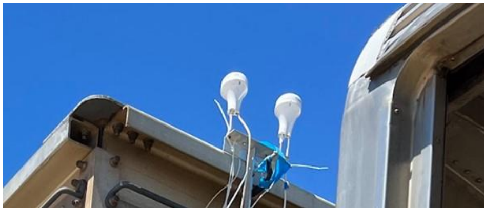
Figure 2-4: The pair of Garmin RS 232 Marine Sensors connected to the top of the freight car
