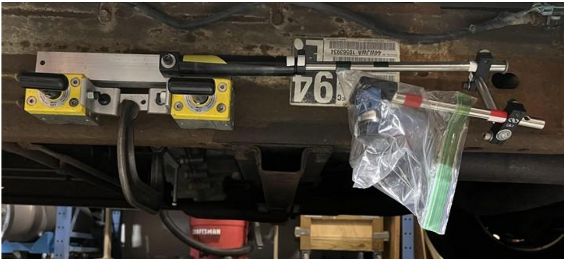
Figure 3-6: Magnetic Lidar test mounting on the lab car frame
