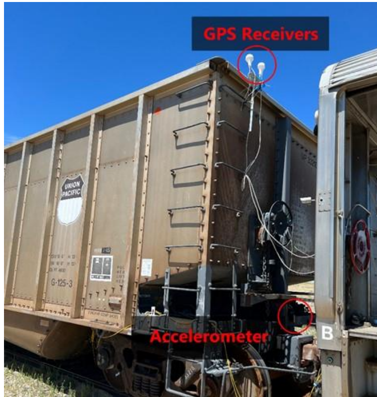
Figure 3-15: GPS receivers and accelerometer mounted to the freight car
