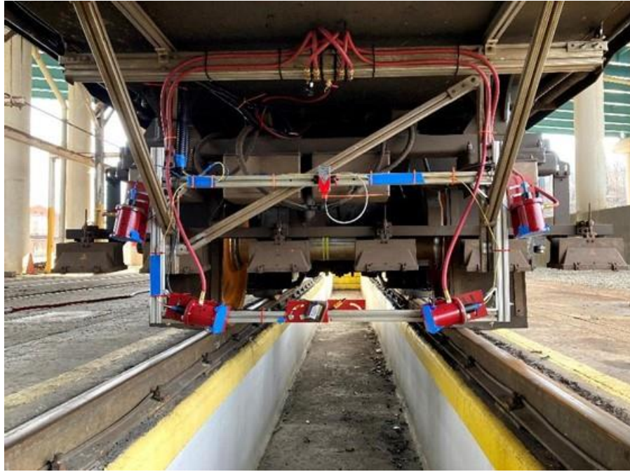
Figure 3-4: Purpose built frame from the 2021 testing attached to the NS 38 track geometry car
