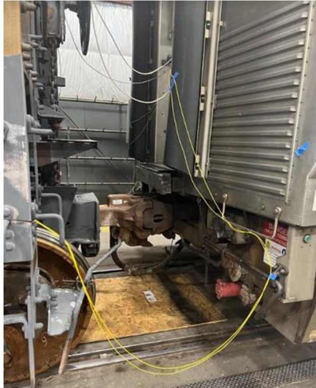
Figure 3-11: Fiber optic cable connected from the rear of the passenger car to the frame of the freight car and down into the wheel well
