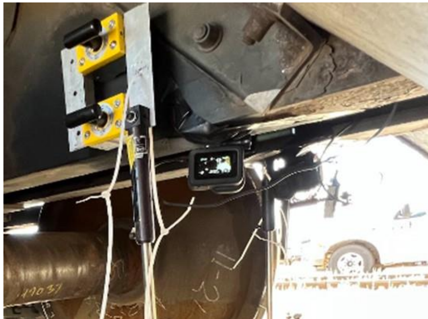
Figure 3-17: GoPro cameras mounted to the center frame of the freight car
