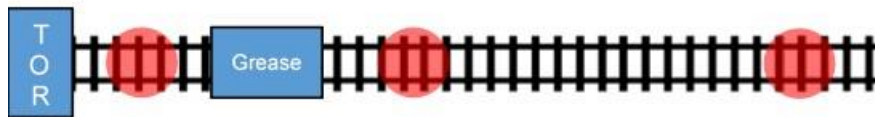
Figure 5-2: Schematic diagram of testing sites (1, 2 and 3), including wayside lubricators. Most traffic is westbound, in this diagram: left to right.
