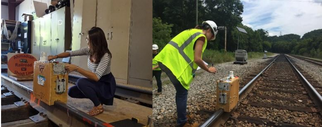
Figure 1-1: Lubricity optical device constructed for this research, used in laboratory testing (left) and validated through field testing (right).
