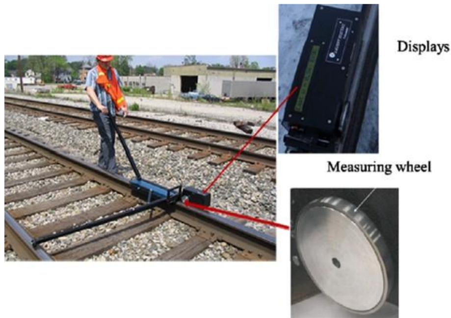
Figure 1-2: Picture of tribometer being used in the rail industry to determine effectiveness of top-of-rail friction modifier material [4].
