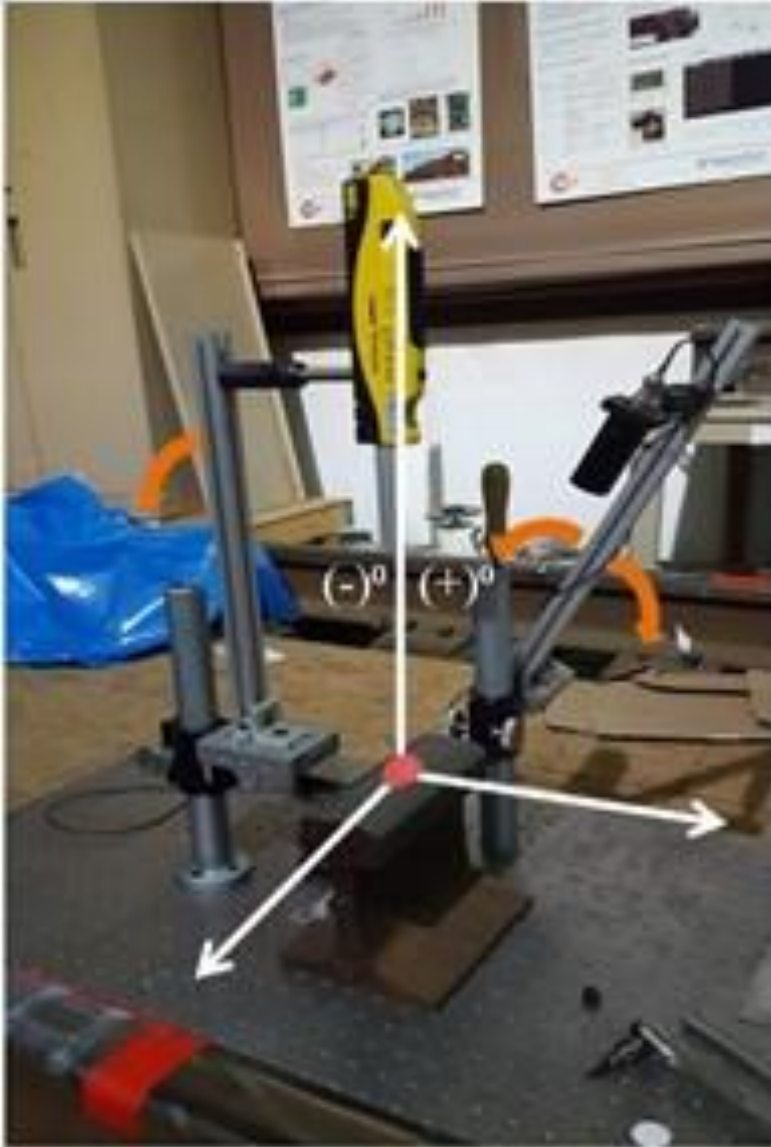
Figure 3-16 shows the experimental setup for out-of-plane measurements. Ambient light and other experimentation logistics were maintained from in-plane experimentation. The emitter included 0^\circ , -30^\circ , -45^\circ , -60^\circ , and -75^\circ increments. Receiver sweeping angle increments consistently ranged from -45^\circ to 90^\circ for the receiver, except for when the emitter fixed directly normal to the rail. These movements were restricted by the physical parameters of the setup.
