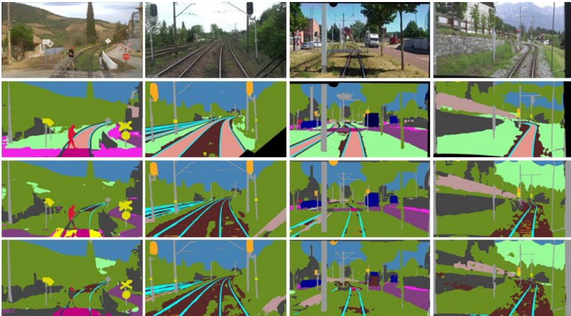
Figure 4.6: Examples of our experiment on the test set of RailSem19 on the selected models. First row = input images; second row = ground truth; third row = output from HRNet + OCR + Multi-Scale Attention; fourth row = output from SFNet(ResNet-18). For the color legend, see Table 4.1.
