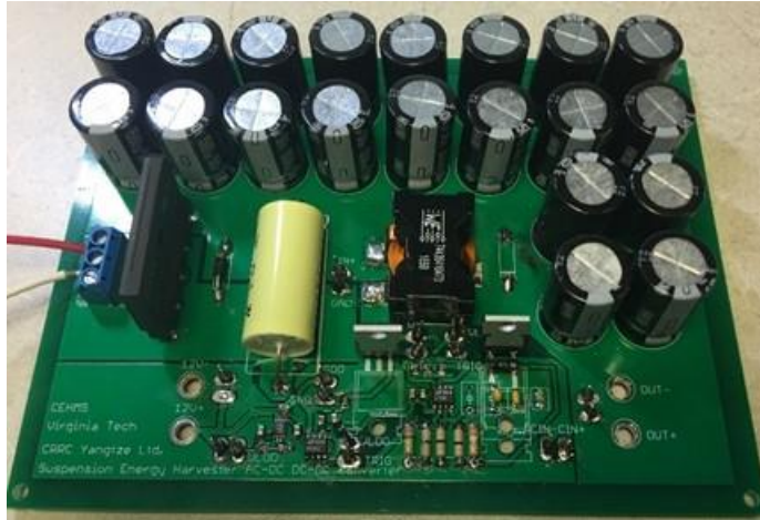
Figure 6-7. PCB of AC-DC and DC-DC (buck-boost) converter
