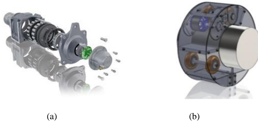
Figure 2-5 Axle generator: (a) FAG Axlebox generator [42]; (b) axle generator with friction wheels [34].
