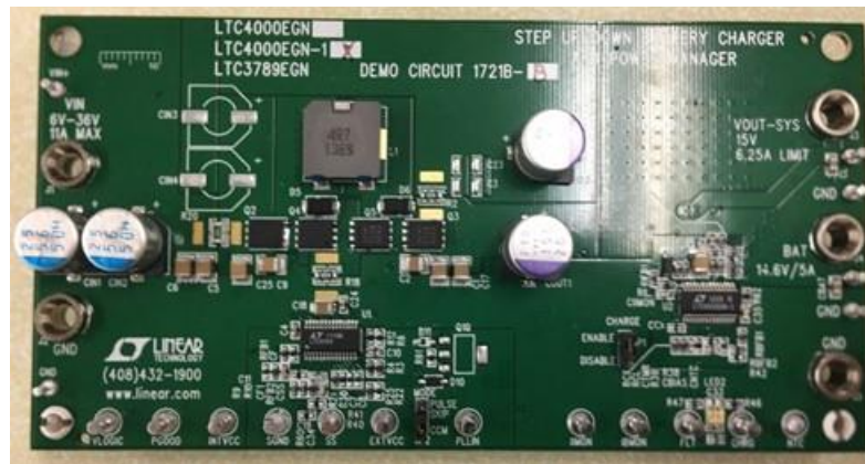
Figure 6-8. Commercial battery charging circuit demo board
