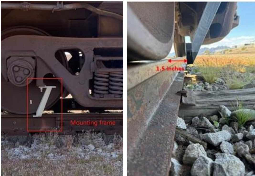
Figure 48 Mounting frame (front and side views)
