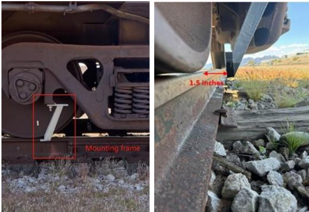
Figure 65 Mounting frame (front and side views)
