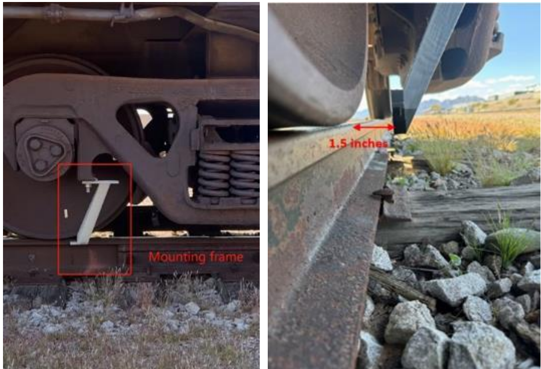
Figure 44. To ensure sensor safety (e.g., not colliding with the rail during the test operation), the sensor was placed 1.5 inches away from the rail head side. Like the rail-mounted test, the sensor location was adjusted from the initial location (Figure 45) by moving it to the far side of the rail by two inches for the subsequent test. A hammer hit was used to synchronize the timeline between the video and the signals, allowing precise synchronization of video and AE signal timestamps and ensuring a detailed downstream analysis.
