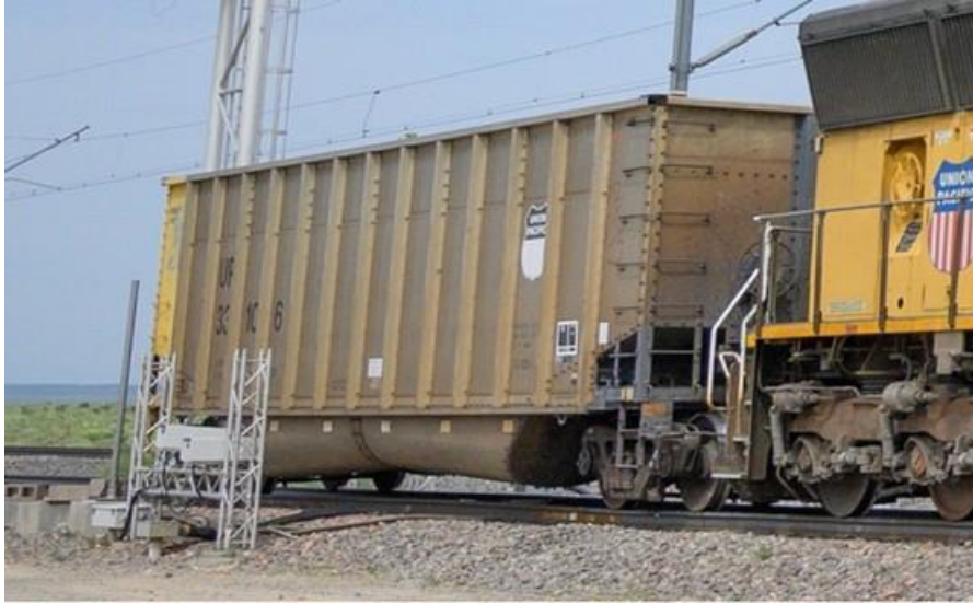
Figure 24 Testing vehicle with 30-ton empty axial load on HTL loop
