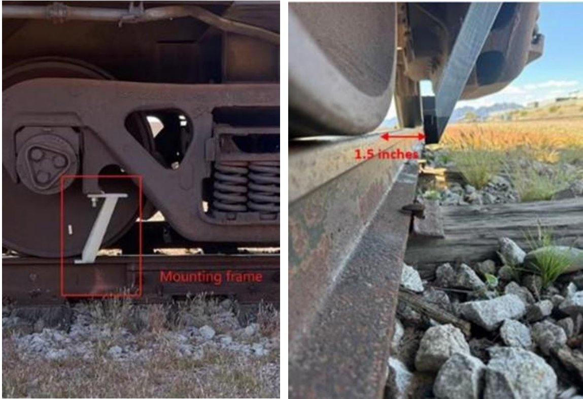
Figure 63 Mounting frame (front and side views)
