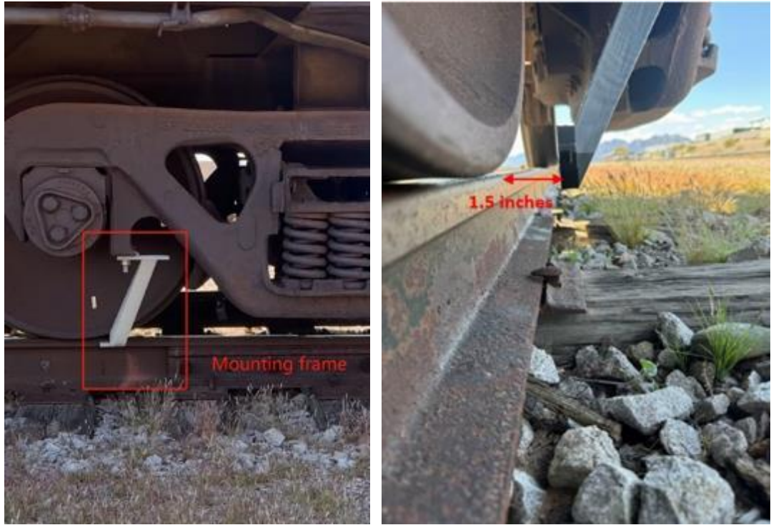
Figure 44. To ensure sensor safety (e.g., not colliding with the rail during the test operation), the sensor was placed 1.5 inches away from the rail head side. Like the rail-mounted test, the sensor location was adjusted from the initial location (Figure 45) by moving it to the far side of the rail by two inches for the subsequent test. A hammer hit was used to synchronize the timeline between the video and the signals, allowing precise synchronization of video and AE signal timestamps and ensuring a detailed downstream analysis.
