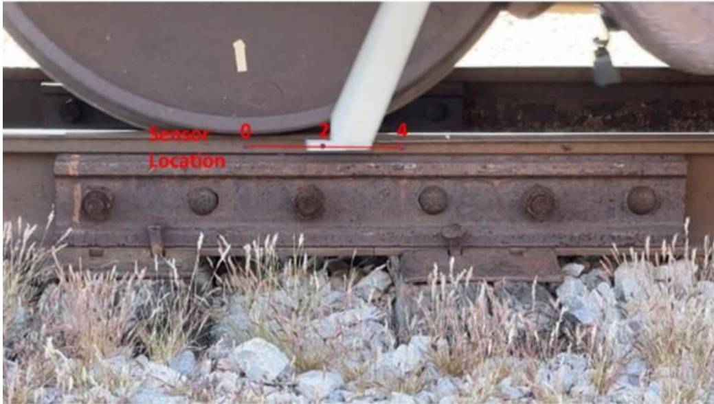
Figure 45 Attenuation evaluation in the rail (longitudinally)
