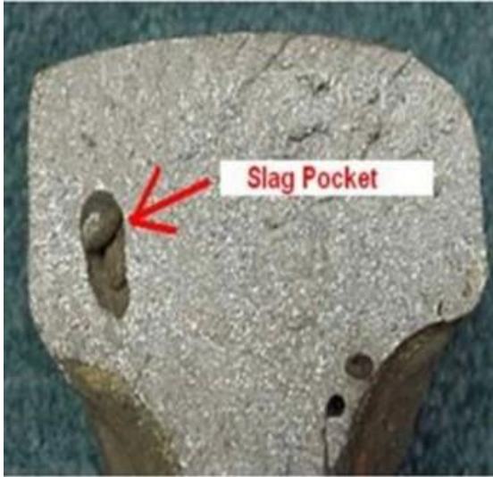
Defective weld with slag entrapment
