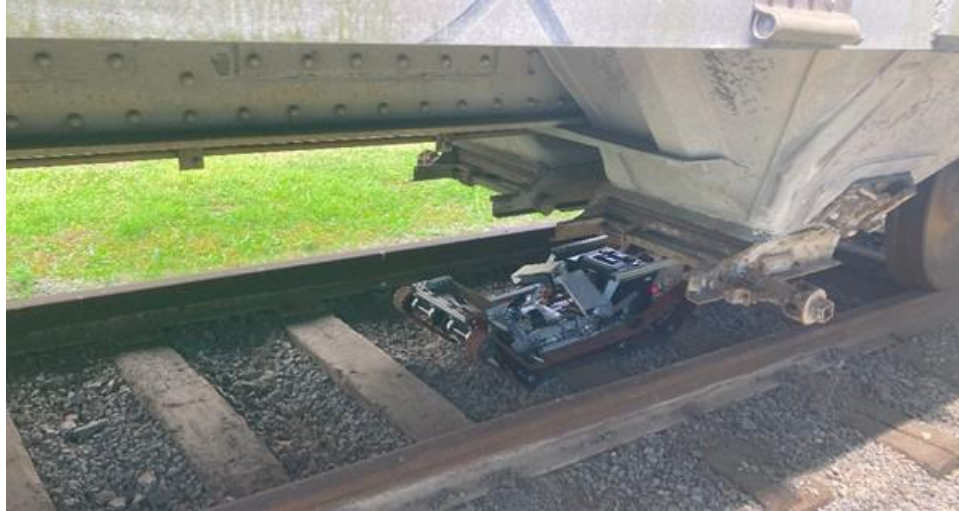
Figure 0-1: The TCR at the testing site, shown beneath the hopper railcar
