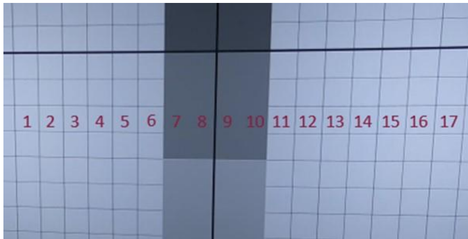
Figure 0-1: This field of view (FOV) evaluation image shows an ability to image only 17 in. wide at a minimum height of 15 in.
