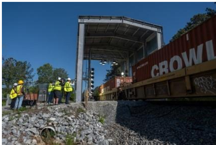
Figure 0-1: A train passes through an advanced inspection portal. Credit: Sofi Gratas/GPB News [6]
