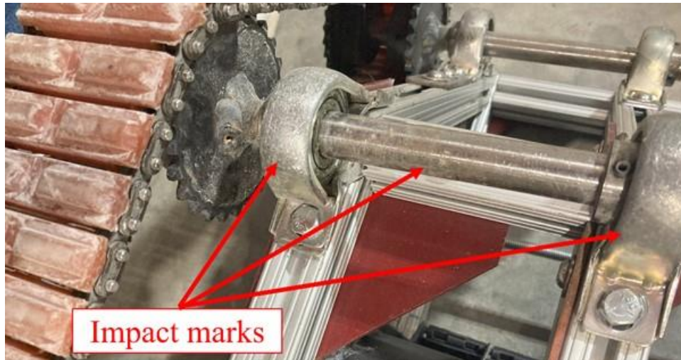
Figure 0-4: Original idler sprocket assembly showing evidence of impacts
