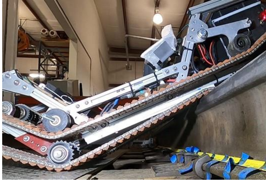
Figure 0-11: Indoor rail climbing test illustrating how the undercarriage plate removes traction from the tracks
