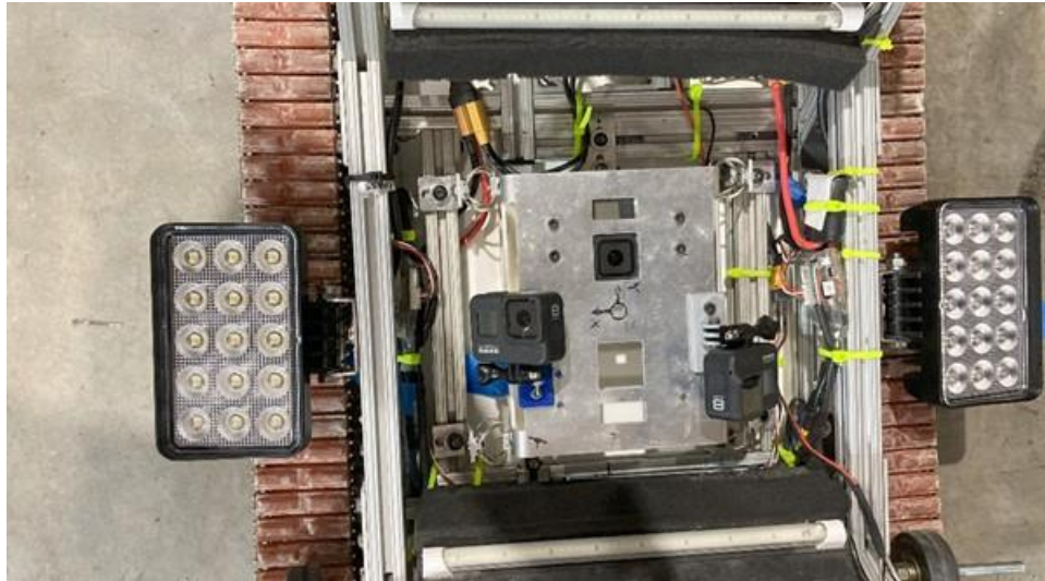
Figure 0-4: Initial configuration of the additional light bars.
