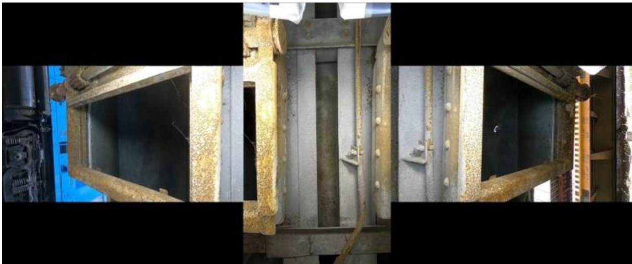
Figure 0-7: Images from the left, vertical, and right-view cameras of a lateral member within the railcar bogie
