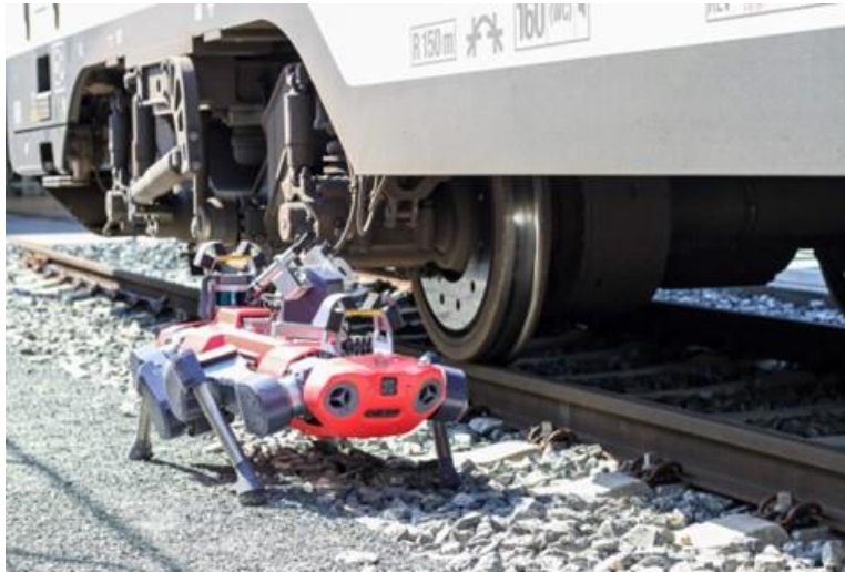
Figure 0-5: The ANYmal conducting an inspection on the side of a railcar. Image reproduced under fair use [40]
