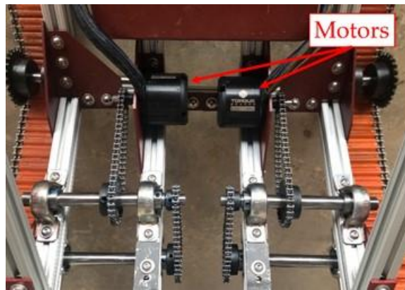
Figure 0-4: The motor and drivetrain components mounted at the rear of the TCR's frame
