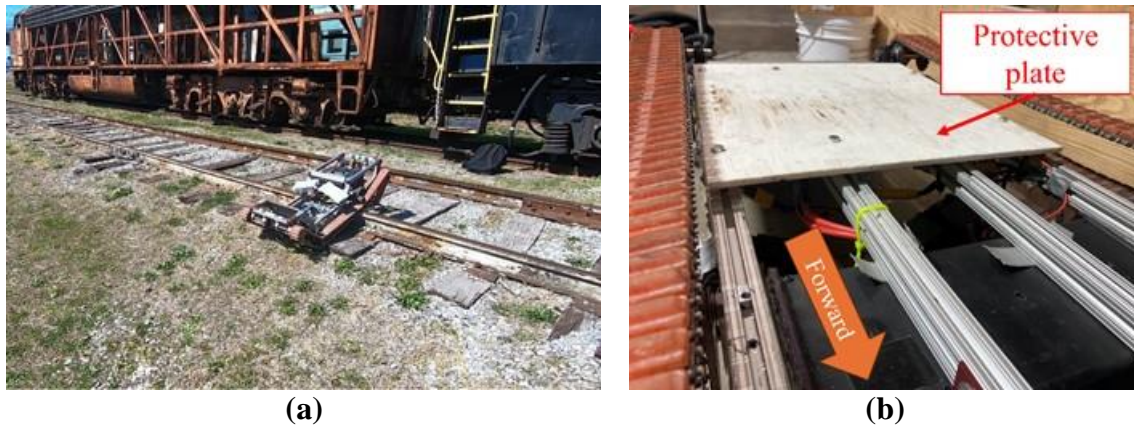
Figure 0-2: (a) TCR shown stuck rail climbing as the edge of the protective plate impacts the rail; (b) the protective plate mounted to the TCR's undercarriage
