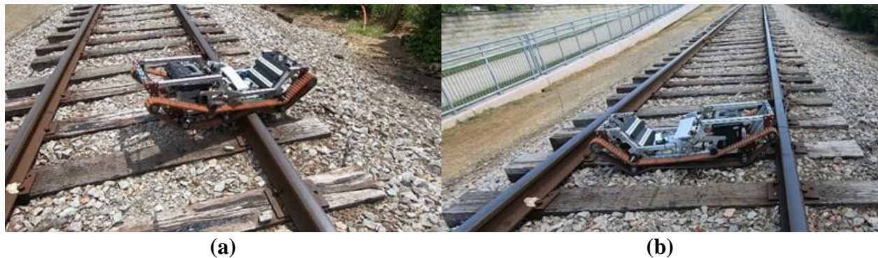
Figure 0-14: Images from the rail climbing test of the improved system: (a) TCR tipping into the track bed while climbing in, (b) TCR becomes stuck on a tie while attempting to climb out
