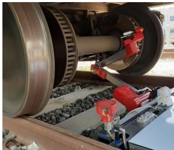
Figure 0-6: The robot developed by Chiaradia et al. [44] inspecting an undercarriage on revenue service tracks. Image reproduced under fair use
