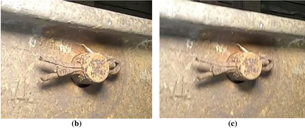
Figure 0-2: Retaining clip on a railcar undercarriage captured at 2 mph using a shutter speed of (a) 1/1920 s., (b) 1/960 s., and (c) 1/480 s.
