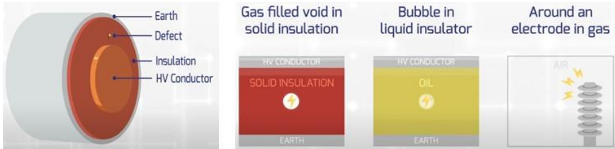
Figure 3 Causes of PD in switchgears and transformers
