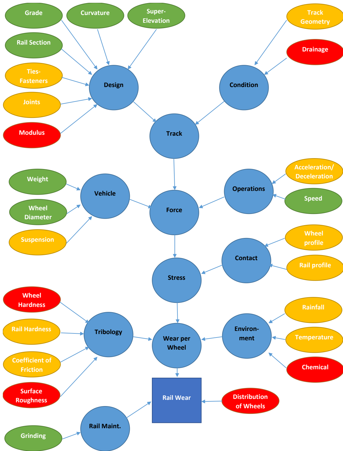
Figure 10 Rail wear flow diagram.
