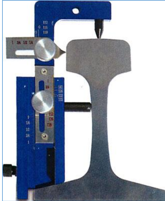
Figure 2 Rail wear gauge (Western Safety Products, 2018)
