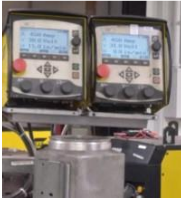
Figure 11.1 ESAB SAW equipment
