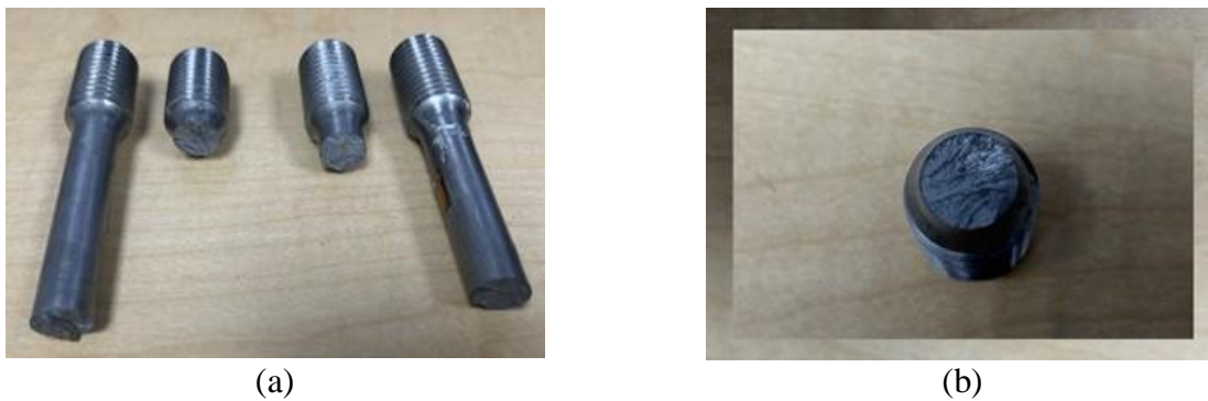
Figure 10.13 Failure shapes of the weld area samples
