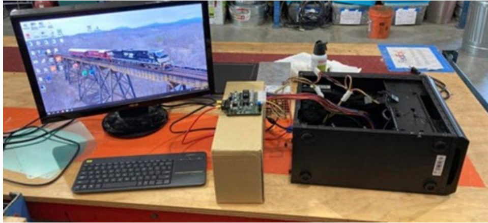
Figure 42: “Fractal” testing under a DC-DC ATGMS compliant power supply
