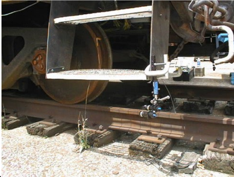
Figure 47: VT Multifunction Doppler LIDAR System Installed on Research Caboose in 2006 using simple C Clamps and Lollipop Mounts
