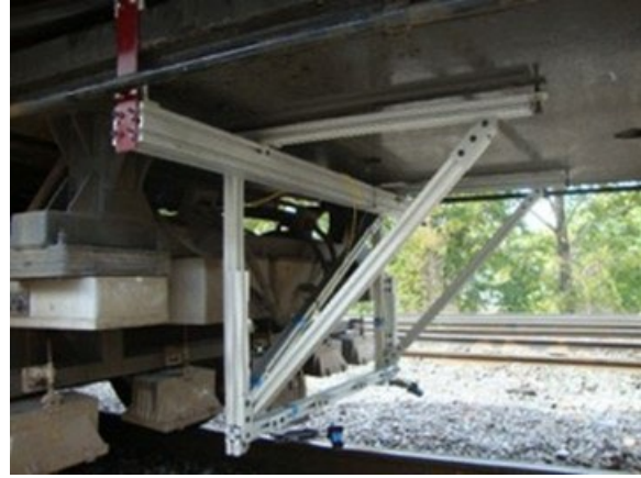
Figure 44: LIDAR Rig on NS 36/38 without explosion-proof housings
