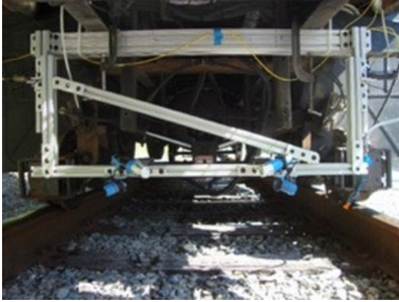
Figure 43: LIDAR Rig on FRA R4 Hy-rail vehicle with multiple lenses installed
