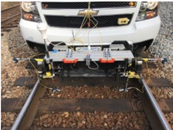
Figure 45: LIDAR Rig installed on NS Hy-rail truck with a mechanical gage sensor
