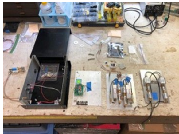
Figure 38: 2020 LIDAR RF unit under construction
