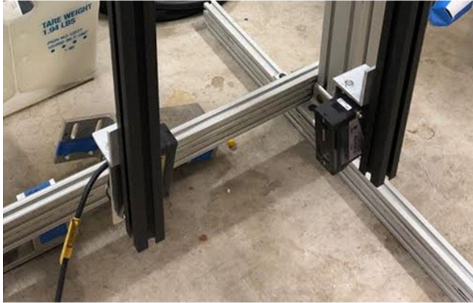
Figure 40: Keyence left and right absolute gage measurement sensors
