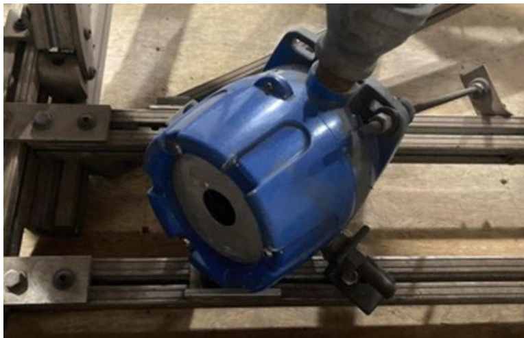
Figure 39: Past 1 in. diameter lens explosion-proof housings with positive pressure air line
