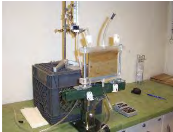
Hydraulic conductivity of a rock slab
